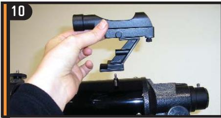
10 Orient the Star Pointer so that the glass window is facing towards the front of the tube. Place Starpointer over the posts on the tube and tighten it down with the knurled nuts.
