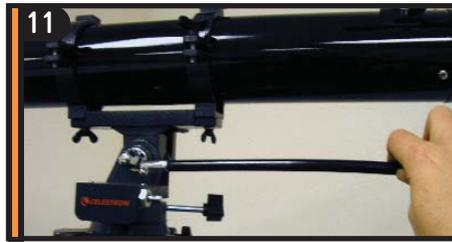
11 Slide the chrome end of the slow motion control cable onto gear shaft and tighten set screw to secure in place.
