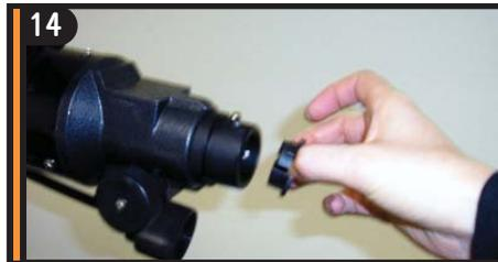
14 Loosen the set screw on the focuser so that it does not obstruct the inner diameter of the focuser. Remove the plastic cap covering the end of the focuser.
