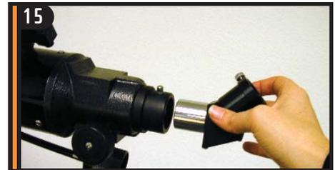
15 Insert the diagonal into the focuser and tighten the set screw.
