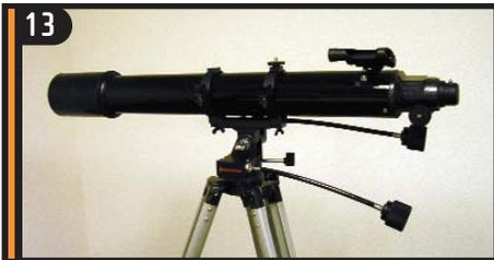
13 Properly assembled, slow motion cables should appear as shown above.
