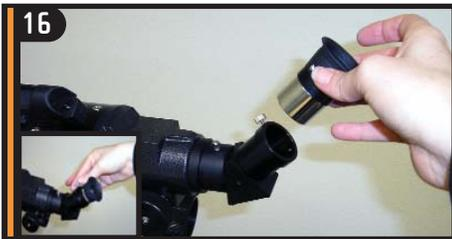
16 Insert the chrome barrel of the 20mm eyepiece into the focuser and tighten the set screw.
