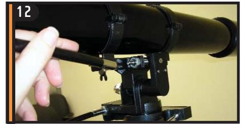
12 Slide the chrome end of the other slow motion control cable onto gear shaft located under tube as shown.
