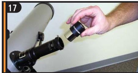
17 Insert the chrome barrel of the 20mm eyepiece into the barlow and tighten the set screw to secure in place.
