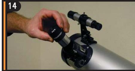
14 Locate the 20mm eyepiece and remove the plastic covers. Insert the chrome barrel of the eyepiece into the focuser and secure in place by tightening the set screw.
