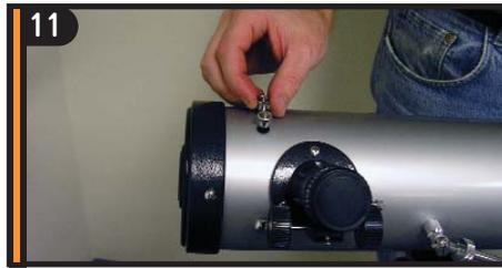
11 Locate the finderscope. Remove the knurled nuts on the threaded posts at the focuser end of the telescope tube.
