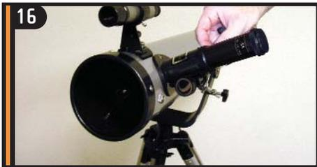
16 For additional magnification, you can use the included 3x barlow. Place the barlow in the focuser in place of the eyepiece and tighten set screw -- remove the cap from the barlow.
