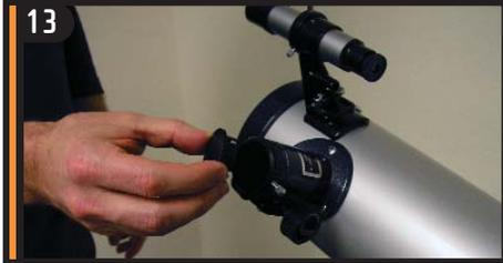
13 Loosen the set screw on the focuser so that it does not obstruct the inner diameter of the focuser. Remove the plastic cap covering the end of the focuser.
