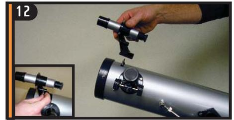
12 Orient the finderscope so that the larger lens is facing towards the front of the tube. Place finderscope over the posts on the tube and replace knurled nuts.
