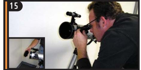
15 Remove the lens cap from the front of the telescope. To observe, look through the eyepiece as shown above.
